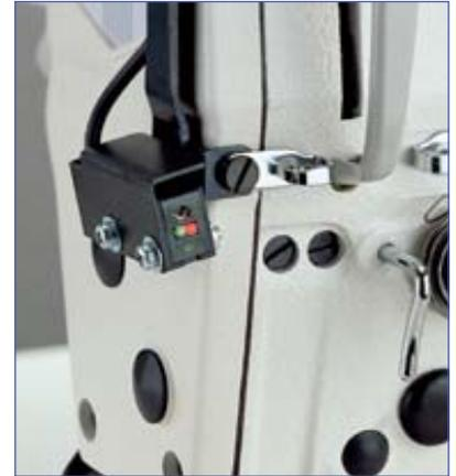
**Newly developed control box/Compact motor unit**
