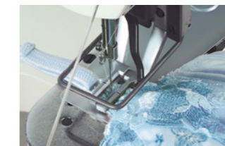
F type (Attaching the shoulder straps to brassier)
