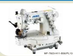
This model is best suited to elastic-band welting for swimwear, briefs, etc. It welts the elastic band which has been overlocked on the garment body.
