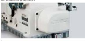
Servomotor Direct-drive motor
