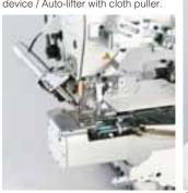
Electromagnetic needle thread / looper thread trimming device
