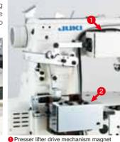
2 Thread trimmer drive mechanism magnet
