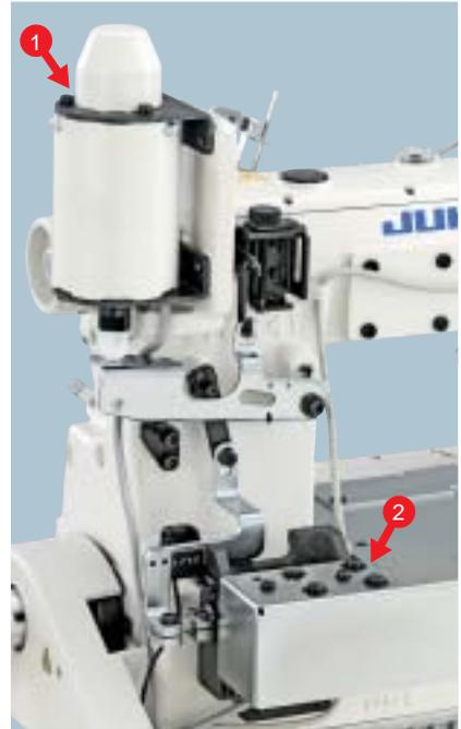
① Presser lifter drive mechanism
