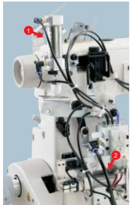
① Presser lifter drive mechanism
