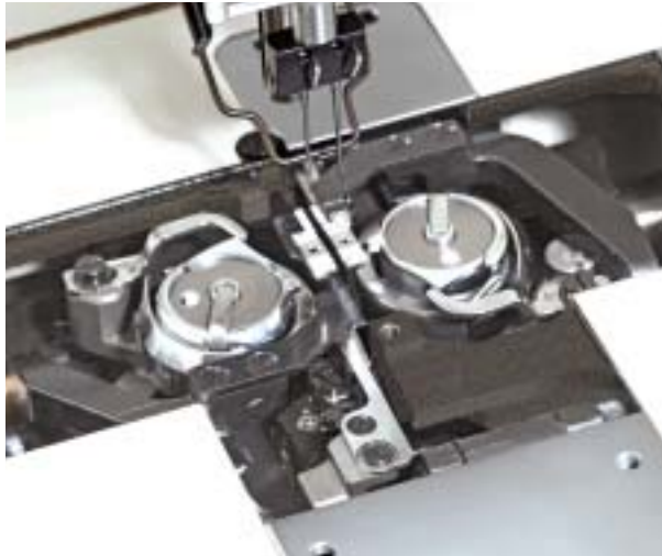
JUKI's unique opener lays down an elliptical locus
