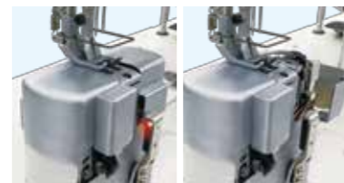
② Hook cover with an open/close sensor
