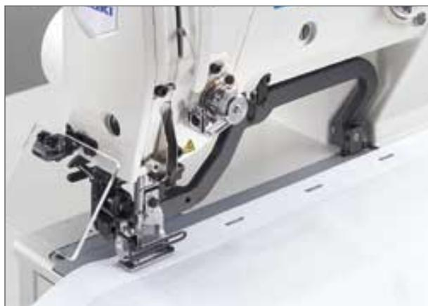
The machine is provided as standard with as many as 30 stitch patterns for buttonholing.
