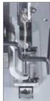
Position of the needle bar during sewing
