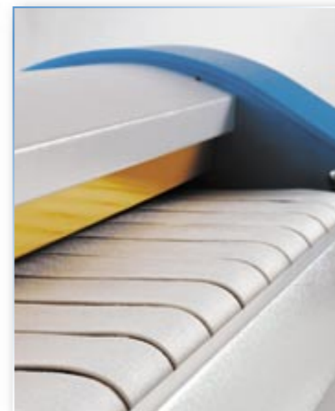
Full-length fingerguard bar positioned and full isolated roller cover
