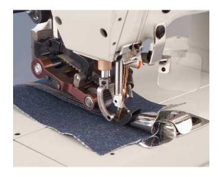
Evenly feed riser and seat plies with a new puller-assisted flatbed lapseamer from Union Special
