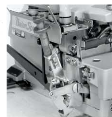
Thumbscrew adjustment for quick setting of gathering ratio.
