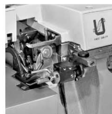
Knee-press controlled stripper blade.
