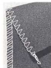
Style 39500 QJ produces two-thread stitch, Type 503
