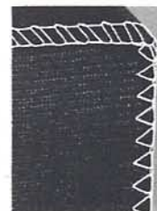
Style 39500 QL produces three-thread stitch, Type 505
